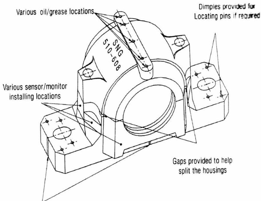
Cross center lines for easy alignment in assembly
